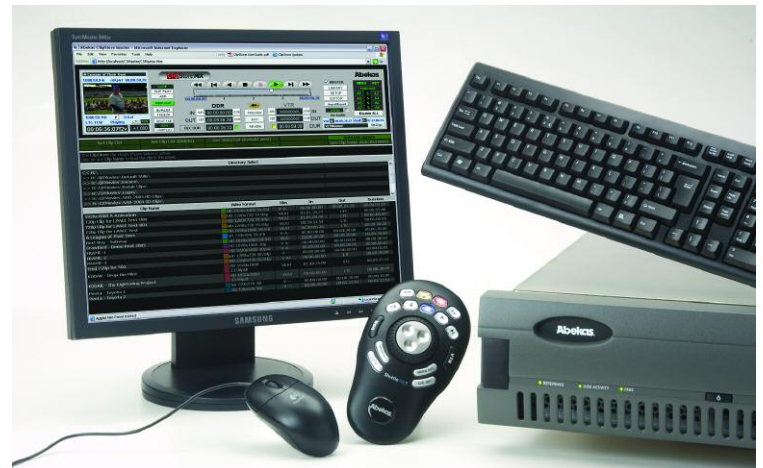
ClipStoreMX system includes ShuttlePRO Control Panel, mouse and QWERTY keyboard.
